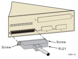
Figure 3-8 2E43-27 or 2E43-27R Straight Cable Connection
